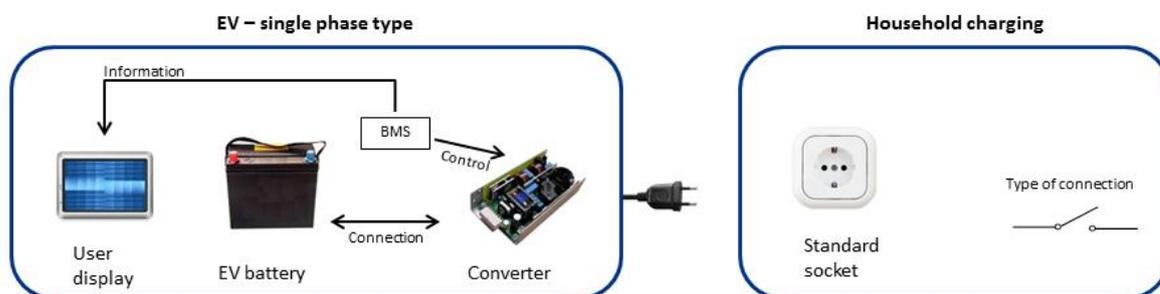
Figure 3.1.1 The battery, converter, BMS and user display in an EV with a connection to a domestic electric socket with an ordinary PCC at e.g. 230V and 10A. This setup falls in charging mode 1.
