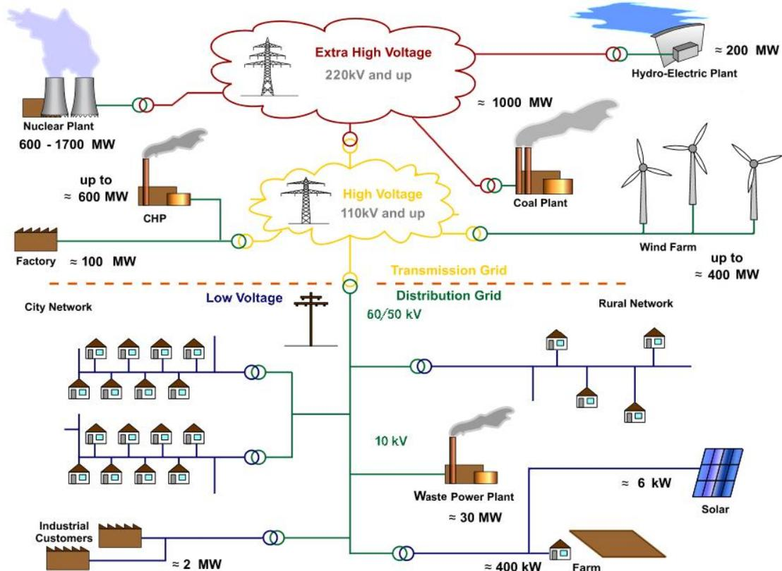
Figure 3.2.1 An overview of the voltage layers (DK) and the general connection levels for various units. The low and medium voltage levels contain the consumers and small scale production while the high voltage grids connect to a variation of production units and particular demanding consumers.
