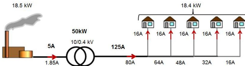
Figure 4.1.5 A small radial with 1 production unit  $P_p$  at 18.5kW and 5 consumers with  $P_c = 18.4 kW$ . The grid loss is 0.1kW in the lines and transformer. The capacity of the transformer is 50kW making the surplus capacity ~30kW. For the radial it is however 45A.
