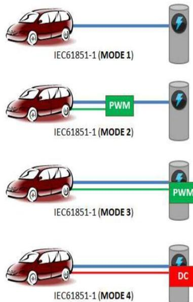
Figure 3.1.2 The 4 different modes of charging according to IEC61851-1
