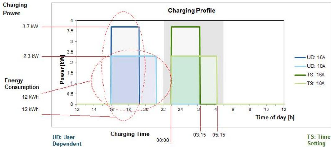
Figure 4.1.2 Shows an example of 4 charging processes with 4 charging profiles for the same EV. The parameters  $S_{ch}$ ,  $E_{ev}$ , and  $T_{ch}$  can be seen as well as their relation and impact on the charge. TS shows the charging profiles shifted to the night time.
