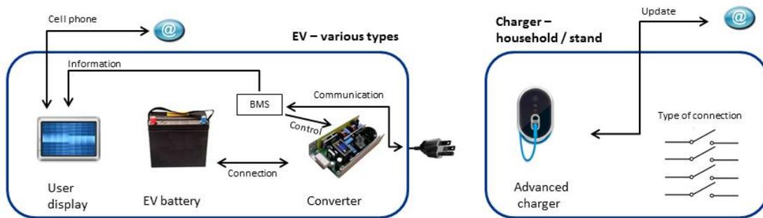
Figure 4.1.1 A simple representation of elements in the EV and charger in an advanced stage of mode 3. The charger has a communication link (Update @) and established three phases plus neutral even if the EV does not require this, yet. The connection includes a communication cable for the charger to agree with the BMS. Information from the EV is possible (Cell phone @) e.g. to the user.
