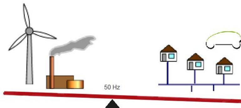
Figure 4.1.4 The production on the left and the consumption on the right must be in balance all the time to avoid negative impact on the grid. Here the frequency is dropping below 50Hz after adding the EV in the residential grid.
