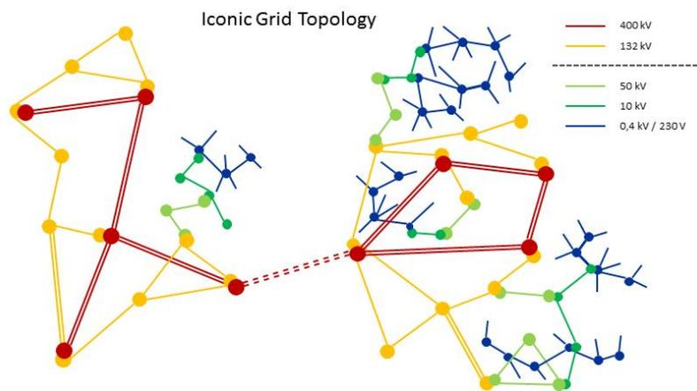
Figure 3.2.2 An iconic overview of the electric system with levels set as in Eastern Denmark. The dashed line is DC which separates the AC areas. Transmission grid has a mesh structure while distribution grid has a radial structure.
