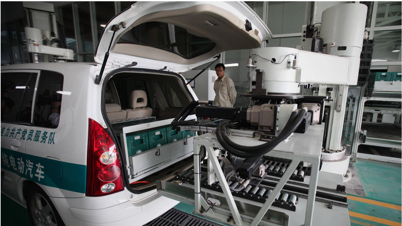
One of State Grid Corporation of China's demonstration projects on battery switching.
