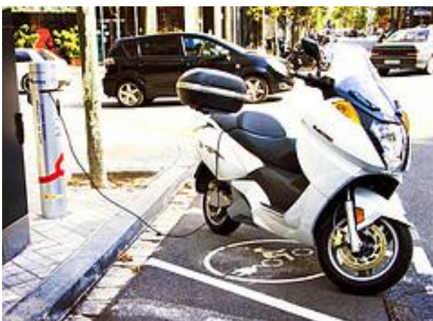
Figure 4.4 - On-street CP for e-Scooters in Barcelona (Source: Live Office 2012)
