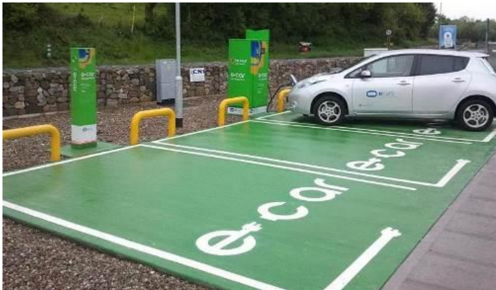
Figure 4.19 – Fully Painted Parking Spaces
