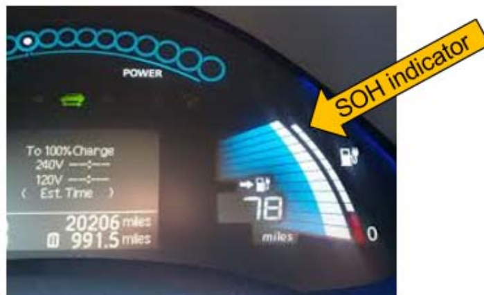
Figure 2.2.2 SOH indicator on a Nissan Leaf
